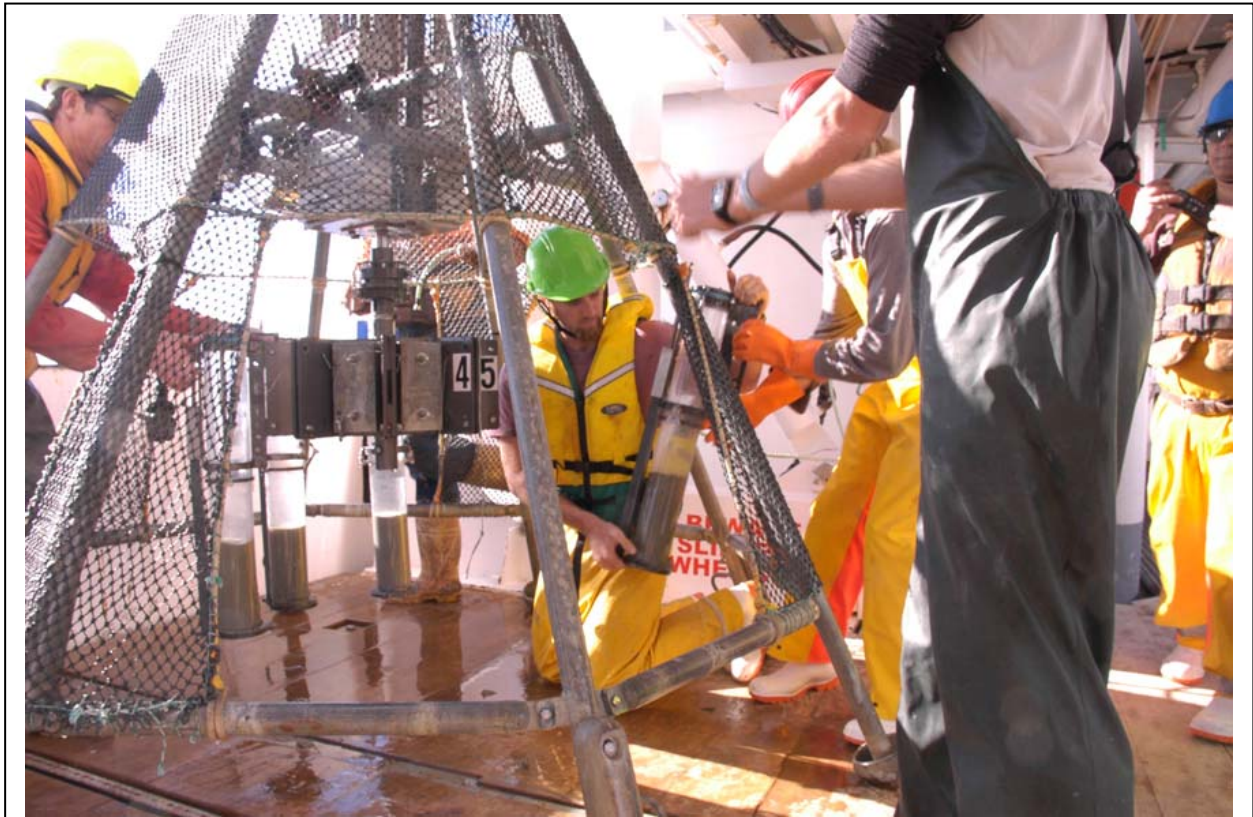
Figure 2: A flurry of activity as scientists unload sediment cores from the multi-corer.
