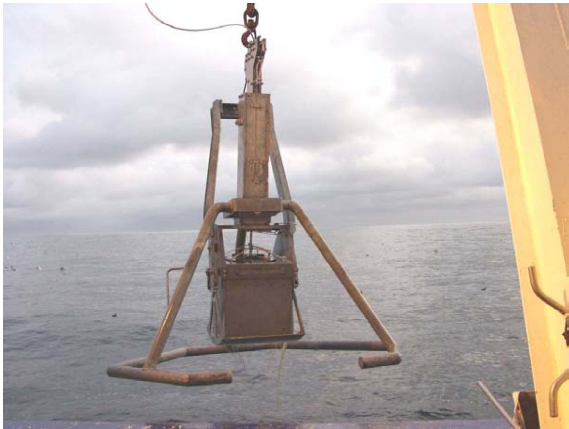
Figure 3: Oktopus box corer being recovered onboard RV Tangaroa .
