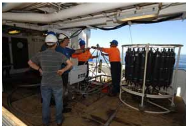
The DTIS (left) about to be deployed during sea trials. The CTD is on the right [Photo: Alan Blacklock, NZ IPY-CAML].
