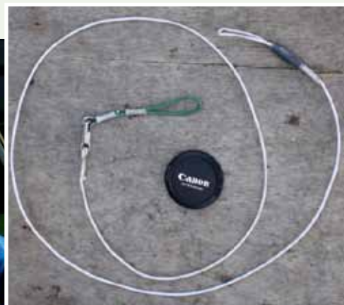
Landing tuna (left) and (above) the winner of this year's Smart Gear competition, Kazuhiro Yamazaki's double-weight branch line. Photos: WWF.
