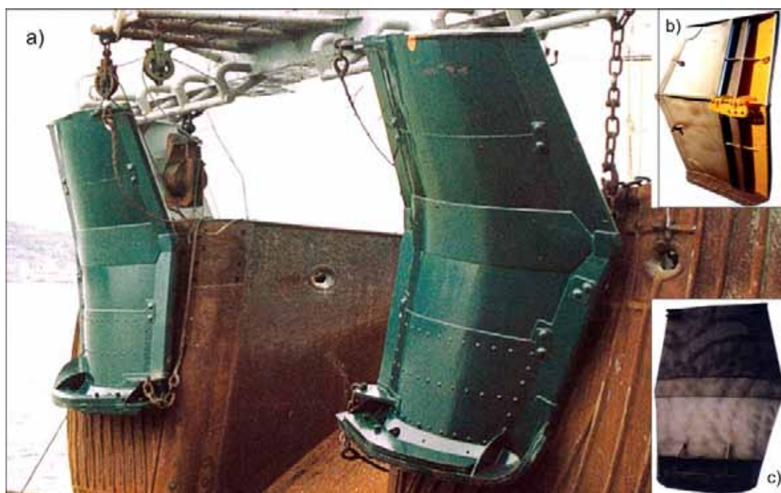
Plate 1. Examples of trawl doors in use on New Zealand deepwater bottom trawlers showing a) Nichimo Super-Vee doors rigged on a trawler stern, b) a Morgere WX door and c) a Morgere WV door.
